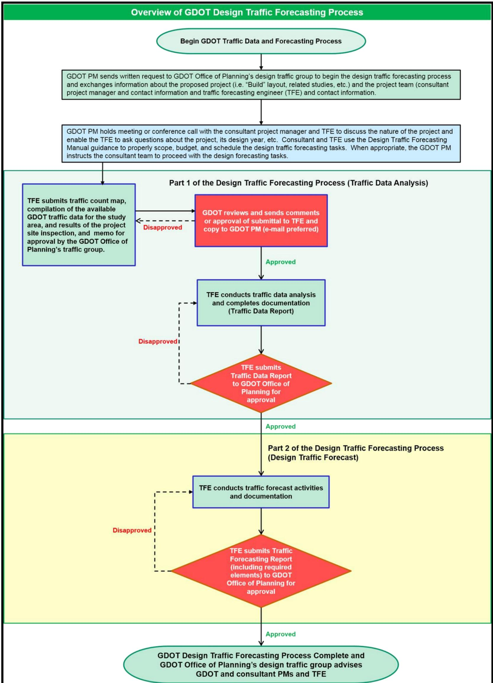
Figure 3.1. Overview of GDOT Design Traffic Forecasting Process
