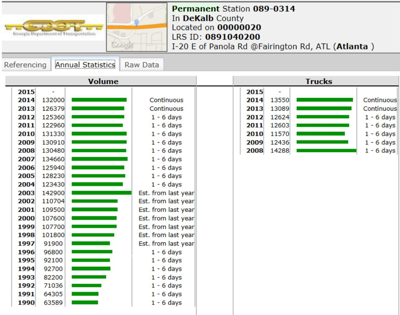
Figure 8.8. GeoCounts – Permanent Traffic Count Stations Sample Data
